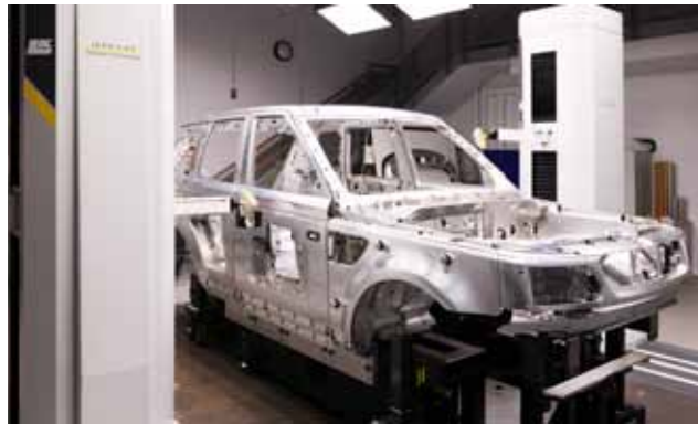
LK H-R premium series twin-rail mounted horizontal arm CMM with walk-on covers
