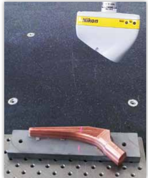
The electrode being automatically scanned.
